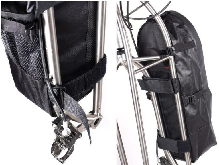
Step 6: Tighten straps on fork legs and make sure hook and loop is securely attached. You may need to readjust the top-attachment strap at this point. Note that there may be excess hook material that needs to be trimmed after final adjustment on upper fork legs. Take a moment to make sure there aren't any loose straps that could get caught in your wheel! Now you can load the packs up and go ride! For more information go to www.jonesbikes.com/support/
