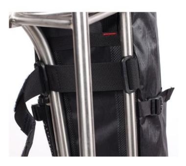
Step 4: Install upper strap from front to rear over the front leg of the truss fork, through the D-Ring at the rear leg of the truss fork, and back through the D-ring at the front leg of the truss fork as shown in the photo below (seen from front in right photo below). The upper strap is now ready to be tightened.
