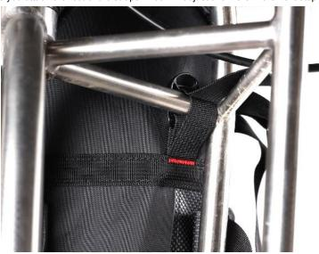
Step 3: Position lower straps. On non-drive side, straps go under the brake hose (left photo below). You may need to adjust the top attachment strap now. Then feed upper strap around front fork leg from front to rear, and through the D-Ring at the rear leg of the truss fork (see inset photo below).
